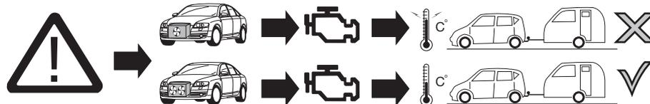
**ATTENTION!** The vehicle's cooling capacity may have to be increased when retrofitting a trailer coupling! You must observe the manufacturer's instructions!!
