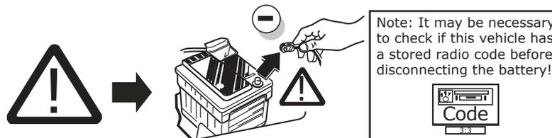
**ATTENTION!** In order to avoid mal-functions and damage to the vehicle's electrical system the earth terminal **must be disconnected** from the vehicle's battery **before starting work!**
